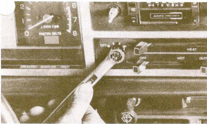
14.4 Removing the nut from the fan control stud (1986 and earlier models)
