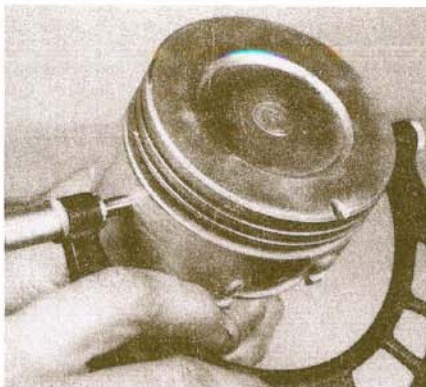
17.11 Measure the piston diameter at a 90-degree angle to the piston pin and in line with it
