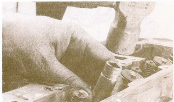
6.2 Gently tap the seal into place with a hammer and deep socket
