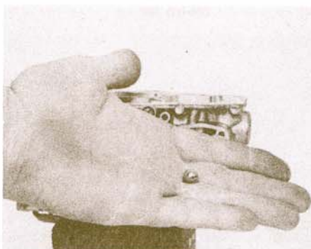
12.26b Anti-overflow mechanism steel ball
