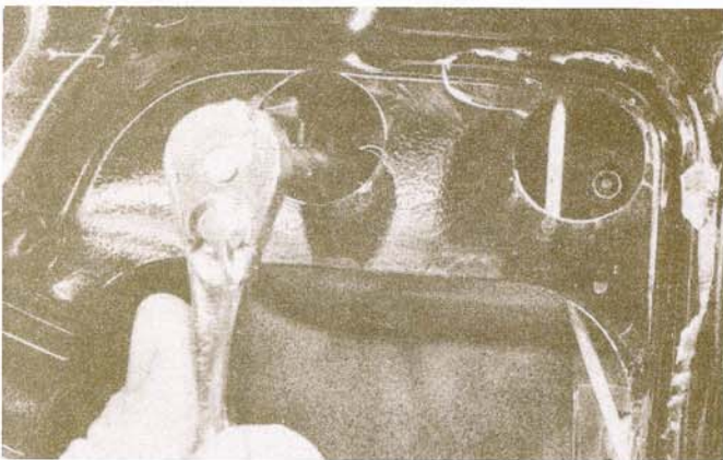
15.8 The exterior handle is attached to the door with two bolts that are accessible from the inside
