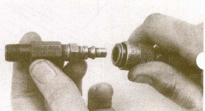
6.4 This is what the air hose adapter that threads into the spark plug hole looks like - they're commonly available from auto parts stores
