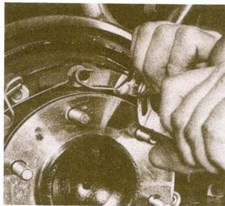
5.4c Remove the forward spring with adjustable pliers
