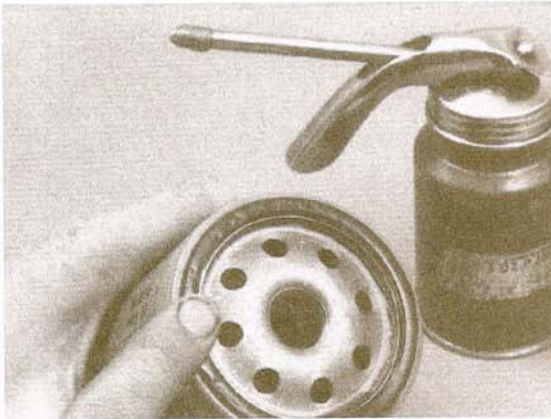
13.18 Lubricate the oil filter gasket with clean engine oil before installing the filter on the engine
