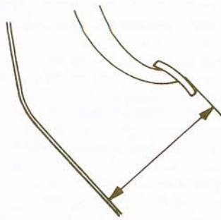
19.2 The clutch pedal height is measured from the top of the pedal to the floor
