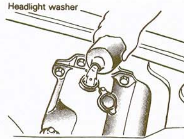
4.14b On headlight washer-equipped models, flip up the cap to add fluid
