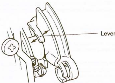
16.61 If the choke valve-to-choke bore clearance is incorrect, bend the throttle lever at the point indicated by the arrows – bending the lever up increases the choke valve-to-choke bore clearance; bending the lever down decreases clearance
