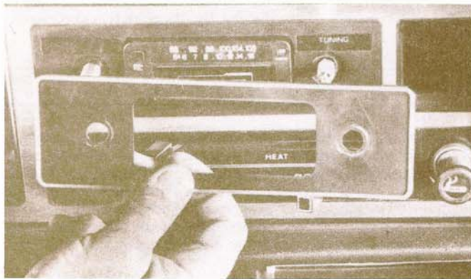
14.3b Removing the radio trim plate (1986 and earlier models)
