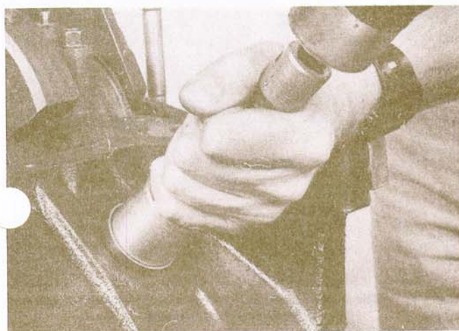
14.10 A large socket on an extension can be used to drive the new core plugs into the bores
