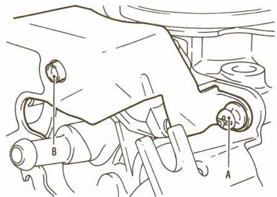
14.37b ... and peen over the heads of the B screws
