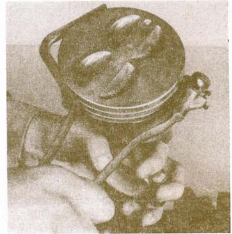
17.4a The piston ring grooves can be cleaned with a special tool, as shown here, . . .
