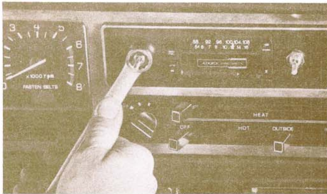
14.3a Removing the radio control stud nuts (1986 and earlier models)
