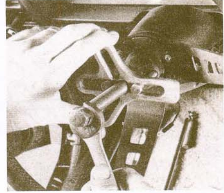
17.6 Remove the steering wheel from the shaft with a puller – DO NOT hammer on the shaft!
