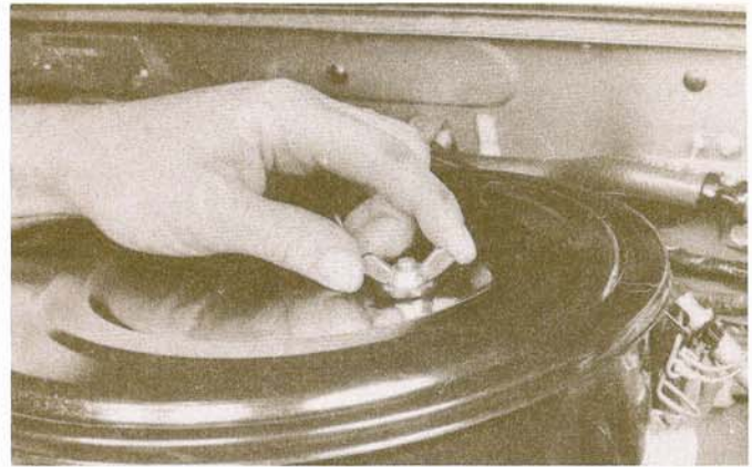
29.3b Remove the wing nut so the top cover can be lifted off
